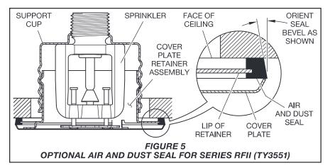
follow this step; otherwise, proceed to Step 8. To attach the air and dust seal, verify the angle of the outside edge of the seal is oriented according to Figure 5. Start the edge of the retainer in the grooved slot of the air and dust seal and continue around the retainer until the entire air and dust seal is engaged.
