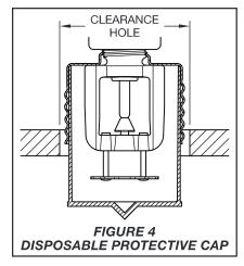
Do not attempt to compensate for insufficient adjustment in the sprinkler by under- or over-tightening the sprinkler/support cup assembly. Re-adjust the position of the sprinkler fitting to suit.
